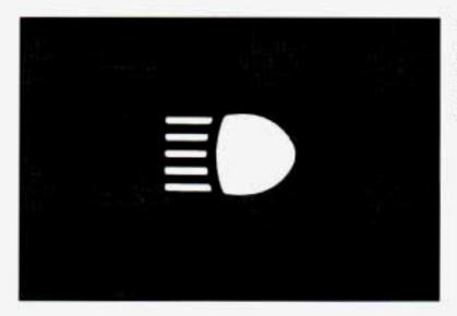
When the high beams are on, this blue indicator light on the instrument panel also will be on.
